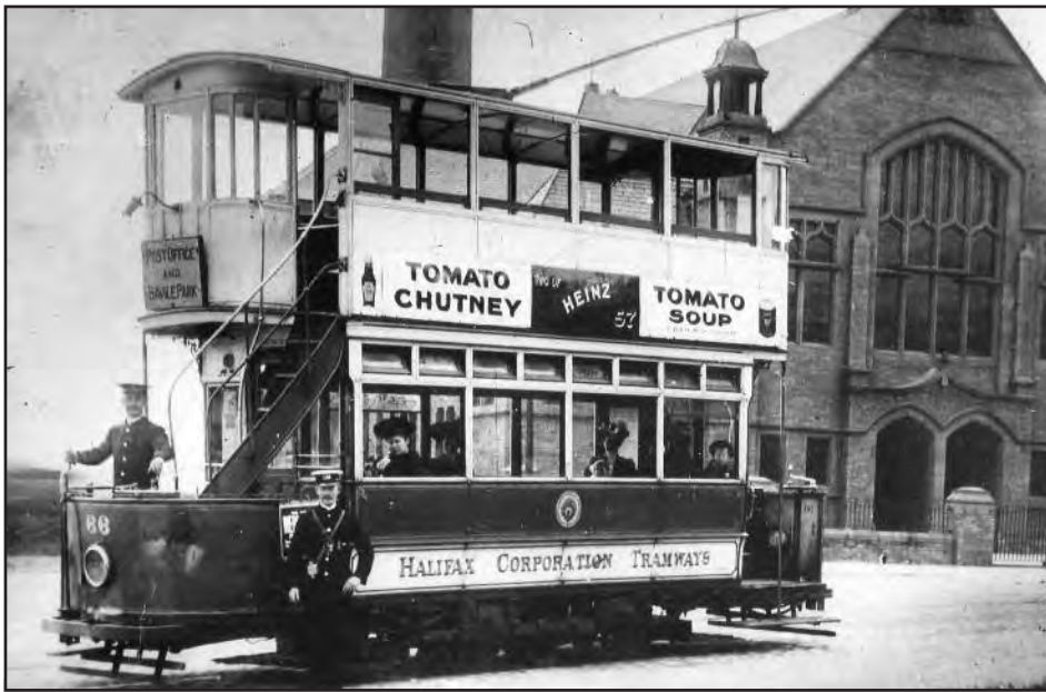
Car 66 displays the early top cover, which it carried from 1906 to 1912. This still left the poor driver totally exposed to the Halifax elements. The tram is standing at College Terrace, the initial terminus of the Savile Park route, just above the school. In the background are King Cross Wesleyan Sunday School and Wainhouse Tower. Heinz already had 57 varieties over a hundred years ago.
